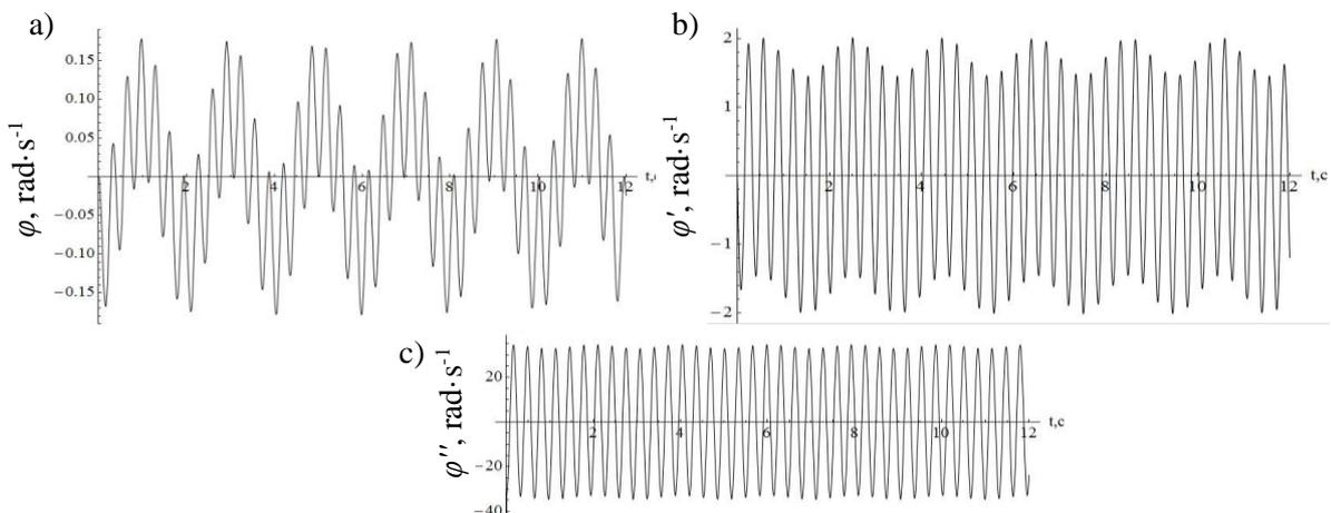
**Fig. 4. Results of the research of dynamics of work of the mobile mixer:** a – schedule of the change of angular movement; b – graph of changes in angular velocity; c – schedule of the change of angular acceleration
