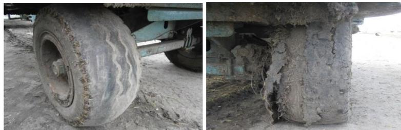
Fig. 1. Wear of the forage mixer wheel tread
