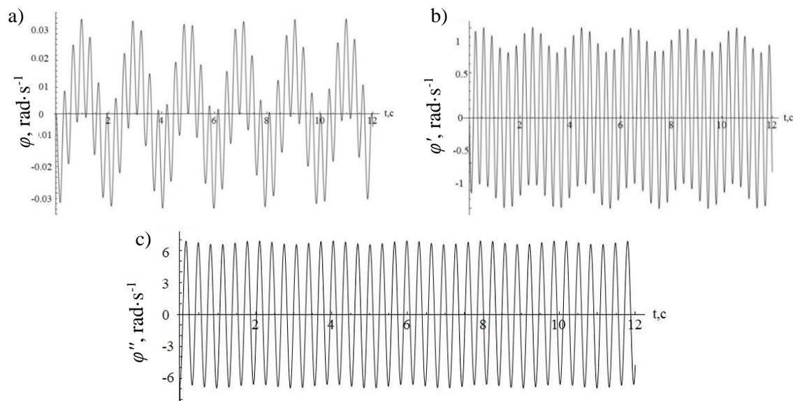
Fig. 7. Results of the study of dynamics of the mobile feed preparation unit: a – schedule of changes in angular displacement; b – graph of changes in angular velocity; c – schedule of changes of angular acceleration
