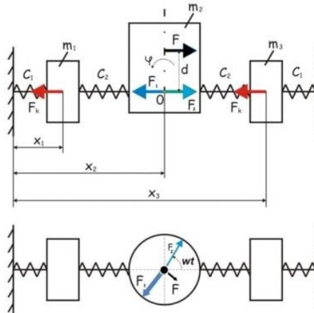
**Fig. 5. Dynamic model of the mobile combined forage preparation unit with the improved working body**
