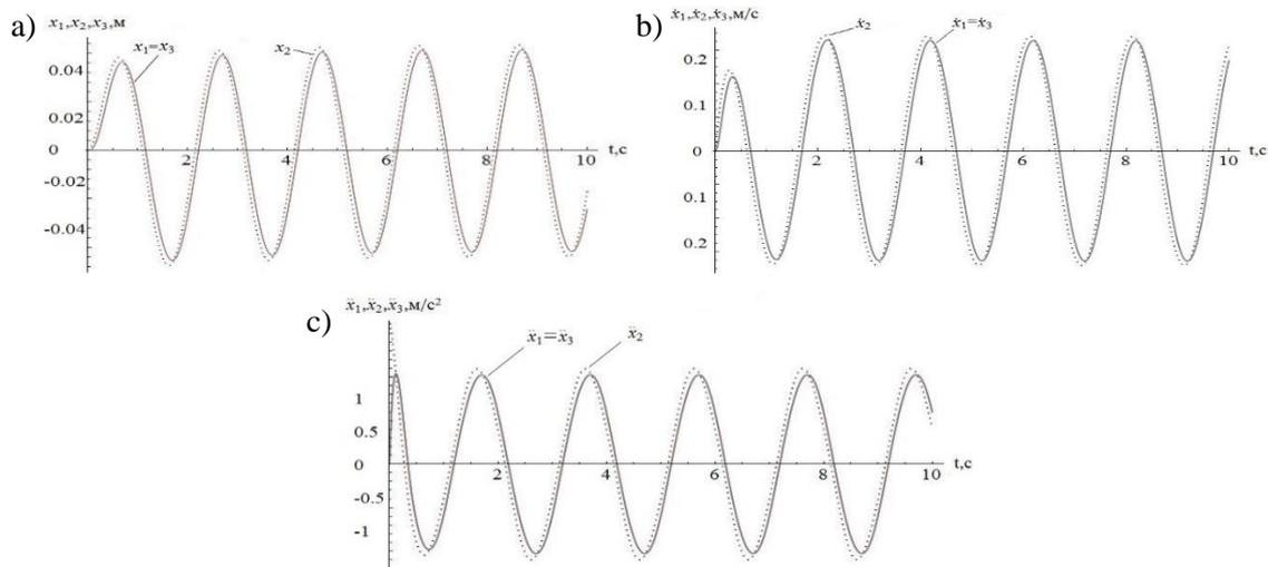
Fig. 6. Results of the research of dynamics of work of the mobile forage preparation unit with the two-western screw working body: a – schedule of movement; b – speed chart; c – schedule of acceleration
